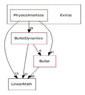
The division of those modules is reflected in Bullet's directory structure, and further subdirectories are provided per module. This means that the Collision Detection module can be used without using the BulletDynamics module.
