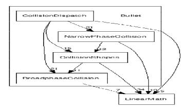
Additional functionality are related to performance and to provide more detail and information useful for the usage in rigid body dynamics and for AI queries in games. The collision pipeline includes 3 stages: Broadphase, Midphase and Narrowphase.
