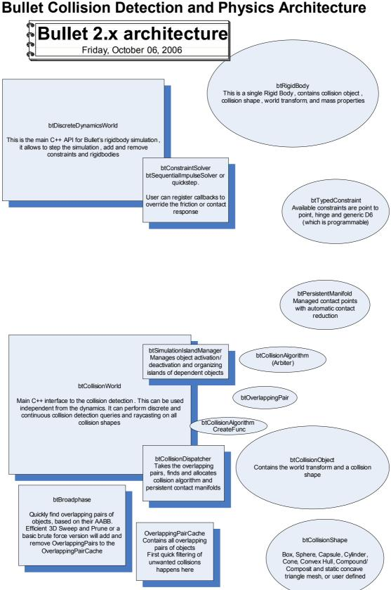
Bullet provides Collision Detection and Rigid Body dynamics. The C++ software is divided into several modules with clean dependencies:
