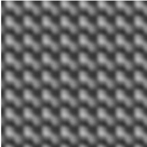
Figure 4.8.9: glm::perlin(glm::vec4(x / 16.f, y / 16.f, glm::vec2(0.5f)), glm::vec4(2.0f));
